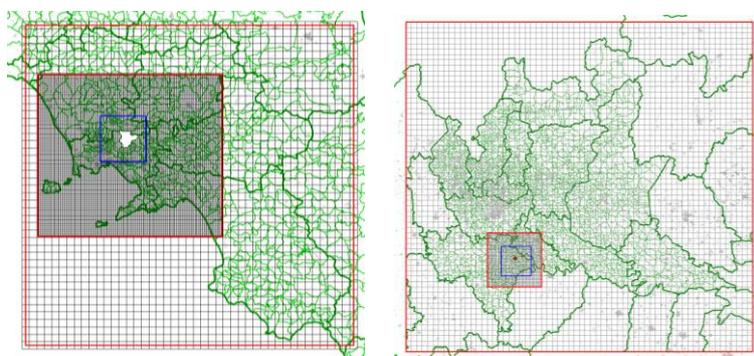
**Figure 1.** Simulation domains: SPRAY "local" domains in blue, FARM "intermediate" and "regional" domains in red
